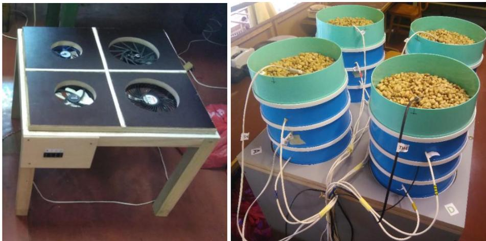
Fig. 1. Laboratory equipment, fan block and wheat drying
