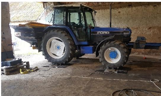
Fig. 3. Measuring of axis weight
