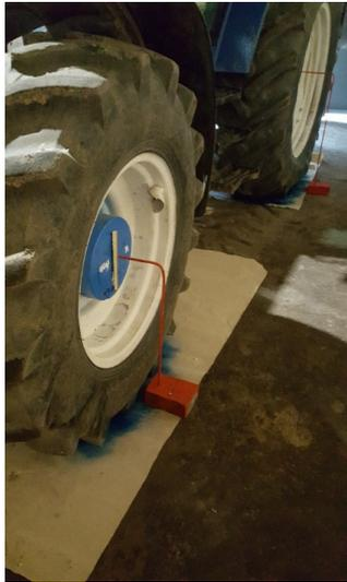
Fig. 1. Measuring of axis height
