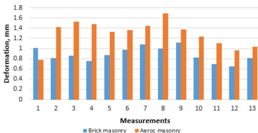
Fig. 10. Measurements of brick and Aeroc masonry samples
