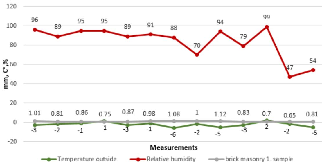
Fig. 9. Measurements of outdoor temperature, relative humidity and brick wall deformation fluctuations
