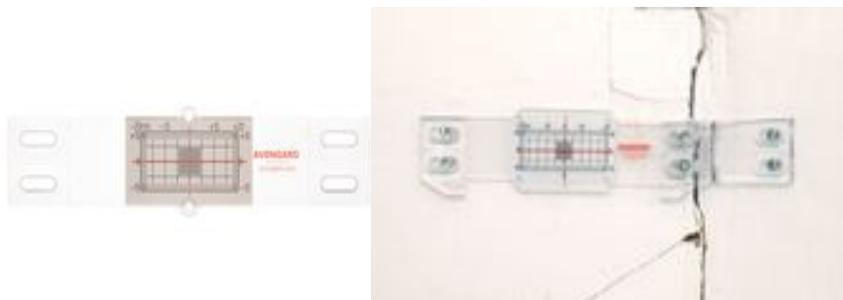
Fig. 1. Standard plane rulers and corner rulers (photo by J.Gruntmanis)
