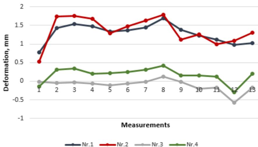
Fig. 7. Aeroc (aerated concrete block) masonry deformation measurements
