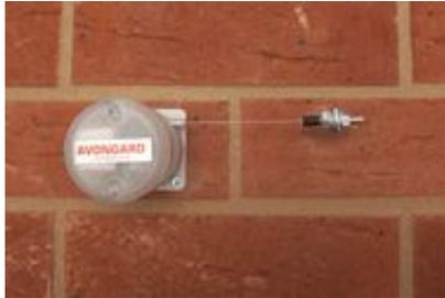
**Fig.3. Digital tools for automatic crack monitoring – electronic data loggers (foto by J. Gruntmanis):** Resolution: 0.003 mm; Range: 80 mm; Linearity: 0.07 % throughout the range; Temperature sensor: -20 till + 80 °C; Resolution: 1 °C; Data capacity: 31926 readings; Power: CR2023 battery; Working temperature: -10 till + 60 °C
