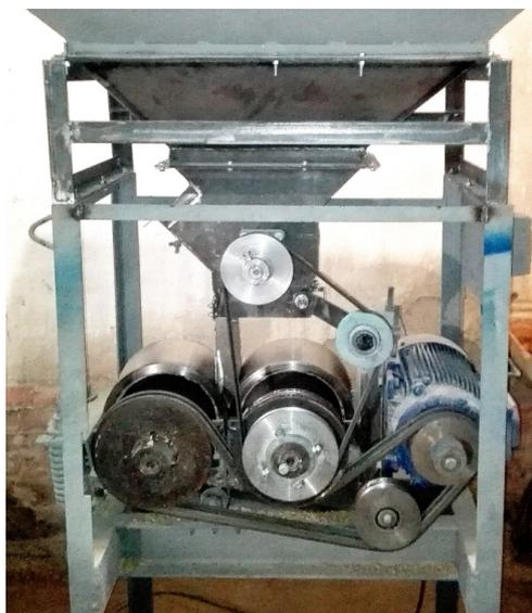
Fig. 3. General view of grain crusher PZ-1M
