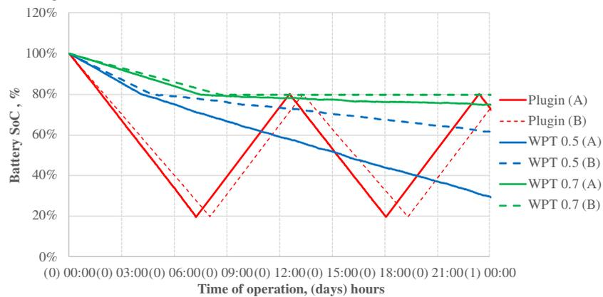
Fig. 9. Battery SoC during 24 hour cycle at various robot charging scenarios
