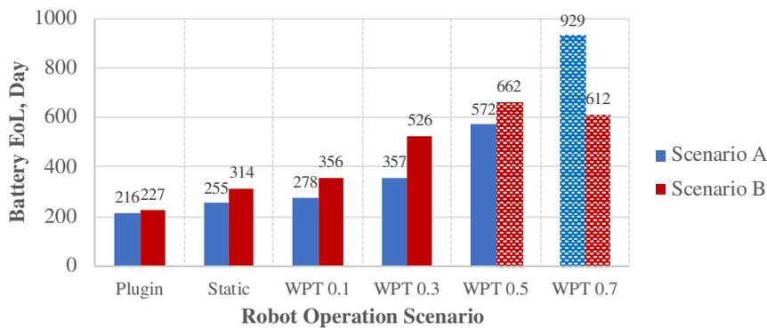
Fig. 7. Battery expected end of life at various robot charging scenarios
