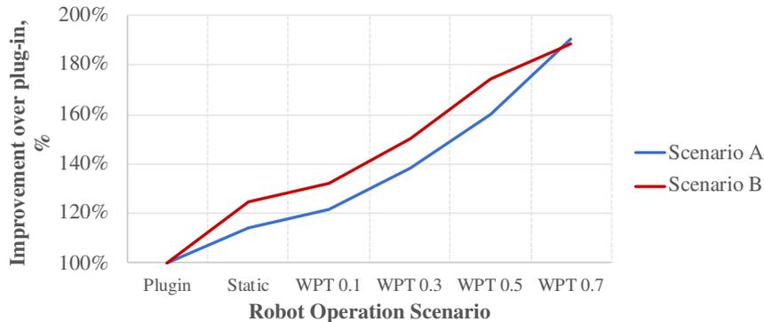
**Fig. 11. Improvement on effective tasks per day at various robot charging scenarios vs plug-in charging**
