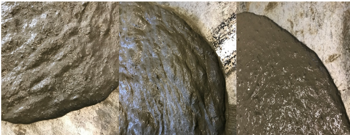
Fig. 2. Cementitious composite spread edge for visual mixture stability assessment, from left to right: M1, M2 and M3
