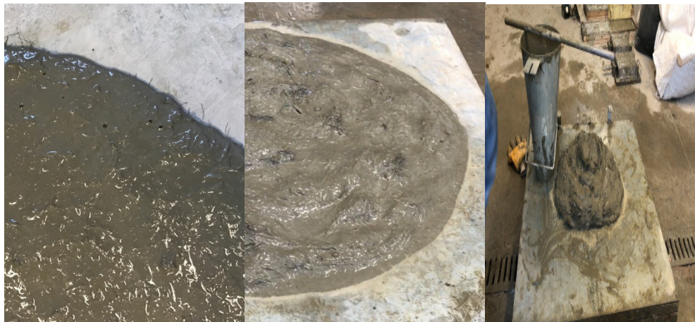
Fig. 3. Cementitious composite spread edge for visual mixture stability assessment, from left to right: M4, M5 and M6
