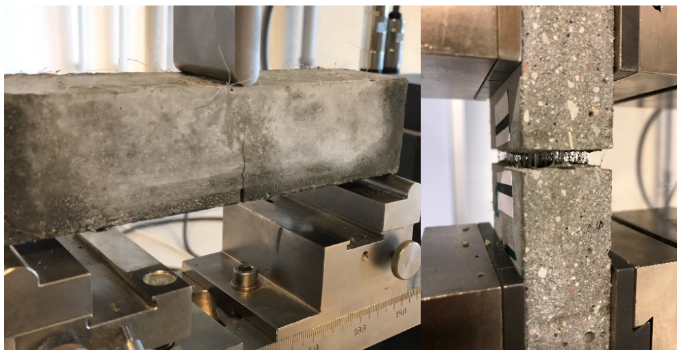
Fig. 1. Single crack bending (on the left) and tension (on the right) test setup
