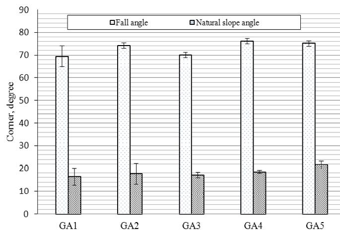
Fig. 3. **Fall angle and natural slope angle of pellets:** GA1 – pure, GA 2 – with molasses add (water and molasses emulsion rate 1:1) ; GA3 – with molasses add (1:2), GA4 – with lime sludge add (1:1); GA5 – with lime sludge add (1:2)
