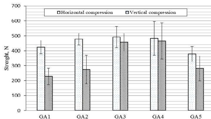
Fig. 2. **Cattle manure compost pellets strength test:** GA1 – pure, GA2 – with molasses add (water and molasses emulsion rate 1:1); GA3 – with molasses add (1:2), GA4 – with lime sludge add (1:1); GA5 – with lime sludge add (1:2)
