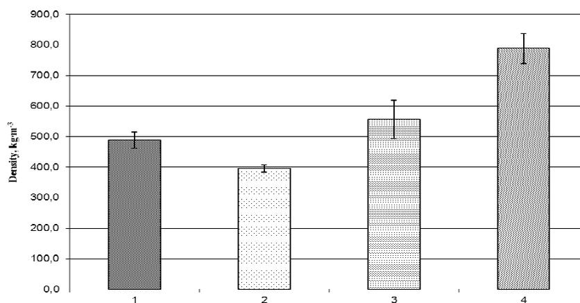
Fig. 1. **Raw material and pellet density comparison:** 1 – naturally dried material density,  $\text{kg}\cdot\text{m}^{-3}$ ; 2 – artificially dried material density,  $\text{kg}\cdot\text{m}^{-3}$ ; 3 – milled material density,  $\text{kg}\cdot\text{m}^{-3}$ ; 4 – pellet density,  $\text{kg}\cdot\text{m}^{-3}$
