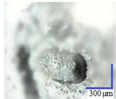
Fig.13. Channel surface left by the oriented fibre at an angle of 80 °
