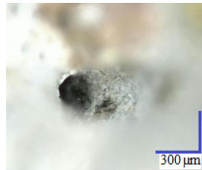
Fig.18. Channel surface left by the oriented fibre at an angle of 10° in sample N55
