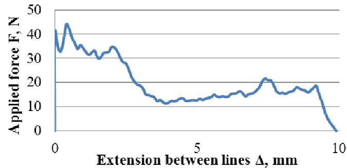
Fig. 5. Pull-out diagram for SF oriented under the angle  $90^\circ$
