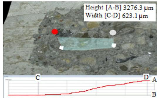
Fig.15. Analysis of channel surface in sample N55 (3D) – 1 part
