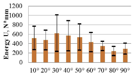
Fig. 20. Average energy of pull-out of one SF at different angle inclination
