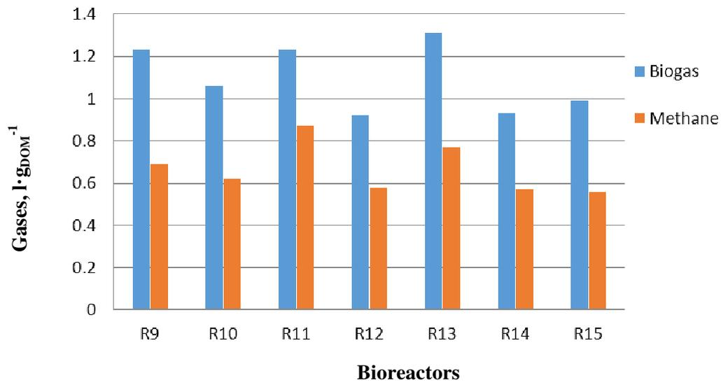
Fig. 2. Specific biogas and methane production from salad beetroots
