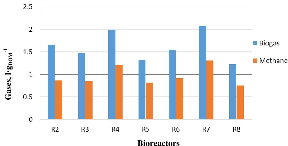
Fig. 1. Specific biogas and methane production from potato crisps
