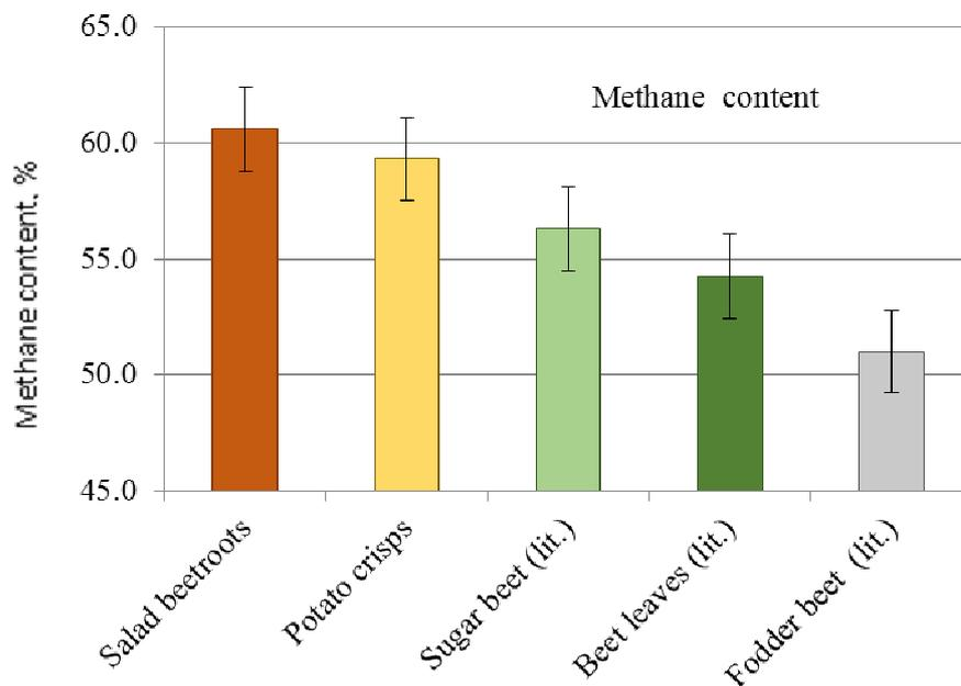
Fig. 3. Methane content in biogas from vegetable wastes: lit. – reference data from literature
