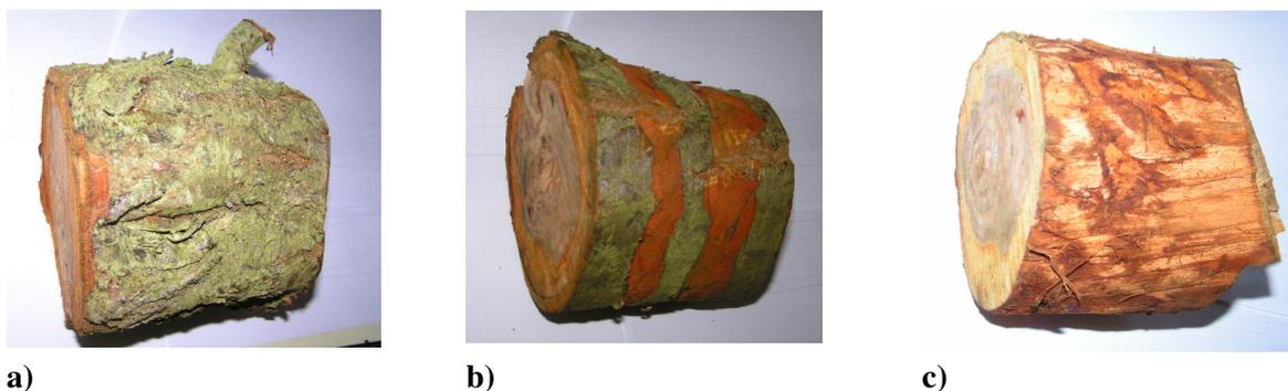
Fig. 1. **Wood big pieces:** a – with bark (100 % of bark); b – with partly removed bark (50 % of bark); c – without bark (bark 0 %)
