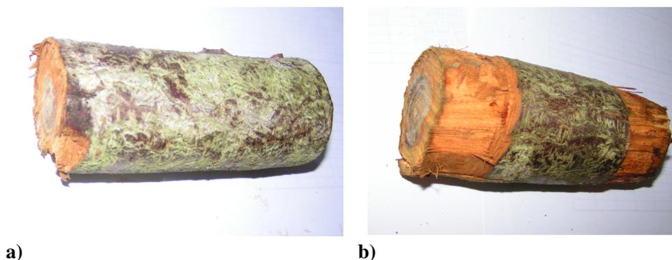
Fig. 2. **Wood small pieces:** a – with bark (100 % of bark); b – with partly removed bark (50 % of bark)
