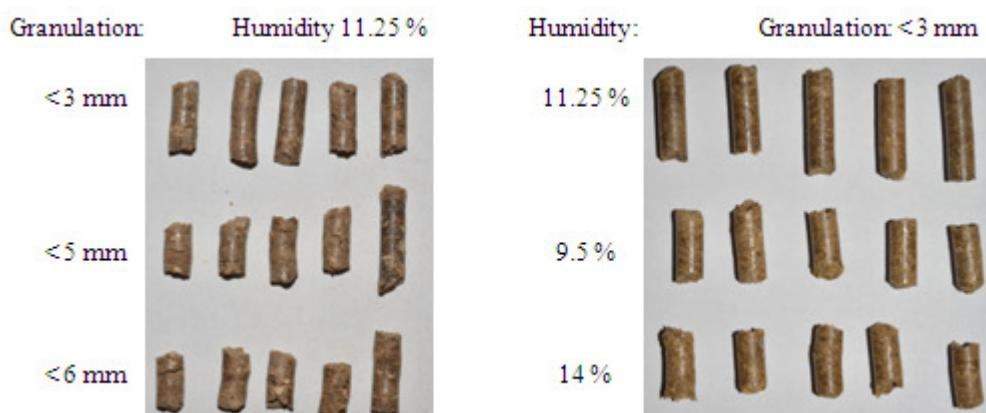
**Fig. 4. Samples of pellets obtained during experiments**
