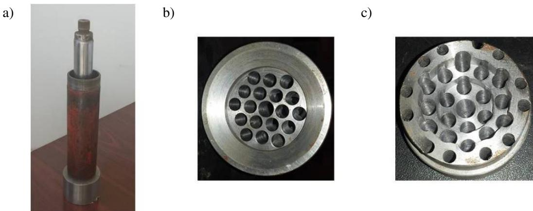
**Fig. 3. Device for compressing biomass at low scale:** a – device ready to be fitted to the force machine; b – 6 mm die; c – 8 mm die
