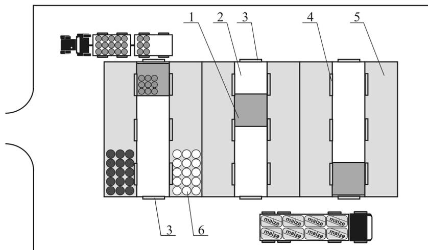
Fig. 1. **Main elements of ASRS:** 1 – elevator cabin with crane; 2 – aisle (shaft); 3 – input/output-points; 4 – pick positions; 5 – racks; 6 – agricultural produce
