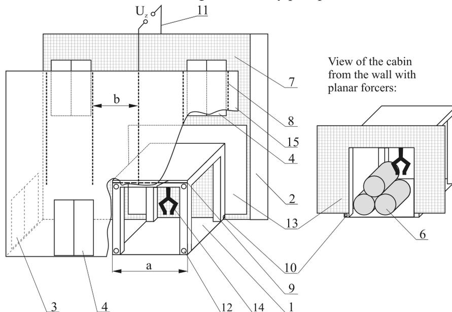
Fig. 2. Main elements of mechatronic rope-free elevator system for ASRS
