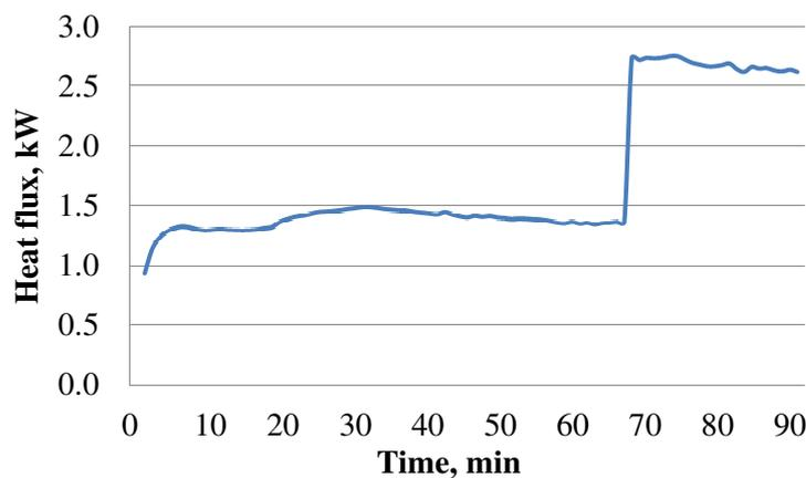
Fig. 4. Heat flux gained from the heat recuperation
