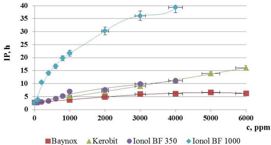
Fig. 3. Antioxidant impact to oxidation stability of RBE
