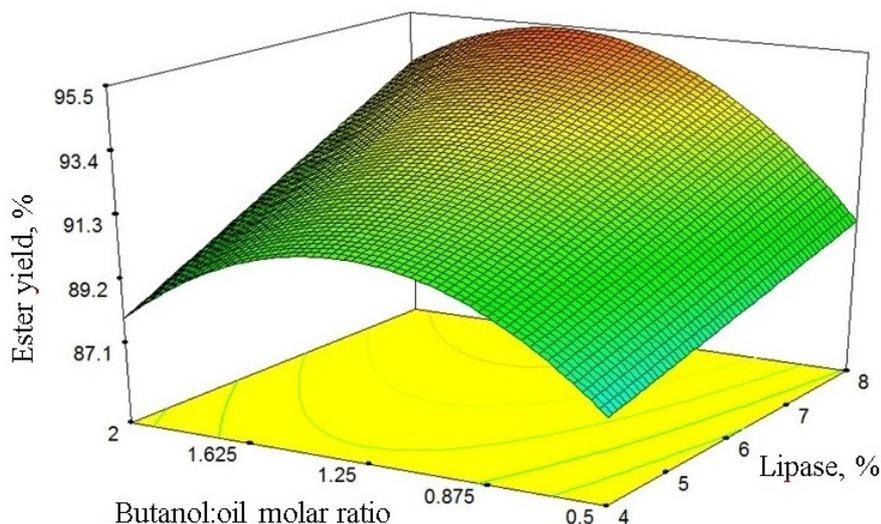
Fig. 2. Response surface plot showing the mutual effects of the butanol and oil molar ratio and lipase concentration on the ester yield of step II, the step II reaction time was 6 hours
