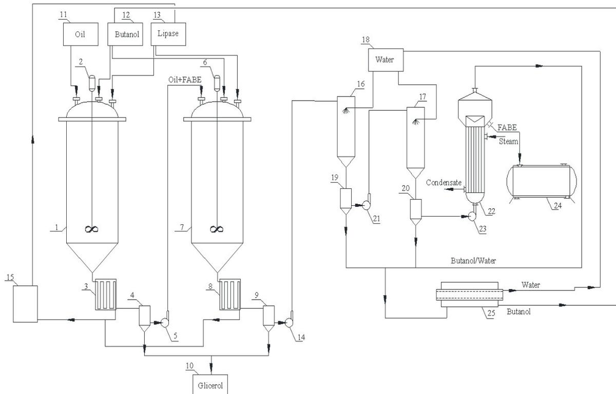
Fig. 4. Principal biotechnological RBE synthesis scheme: 1, 7 – transesterification reactors; 2, 6 – mixers; 3, 8 – filters; 4, 9, 19, 20 – settlers; 5, 14, 21, 23 – pumps; 10 – glycerol collection tank; 11 – oil tank; 12 – butanol tank; 13 – lipase tank; 15 – lipase regeneration; 16 – first washing; 17 – second washing; 18 – water tank; 22 – film evaporator; 24 – RBE tank; 25 – butanol/water separator
