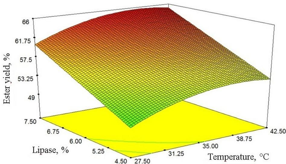
Fig. 1. Response surface plot showing the mutual effects of time and temperature on ester yield, the butanol and oil molar ratio was 3, and the reaction time was 9.75
