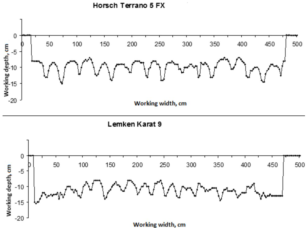
Fig. 4. Furrow bottom profile – row chisel tillers
