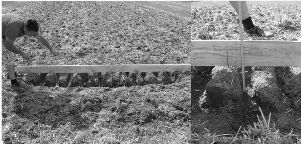
Fig. 1. Furrow bottom profile measurement
