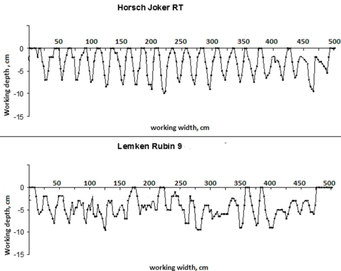
Fig. 5. Furrow bottom profile – disc tillers
