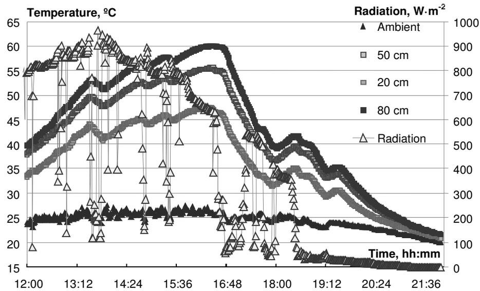
Fig. 3. Radiator water temperature variations depending on solar radiation and distance from air inlet in collector (A, B, C from Fig. 2)
