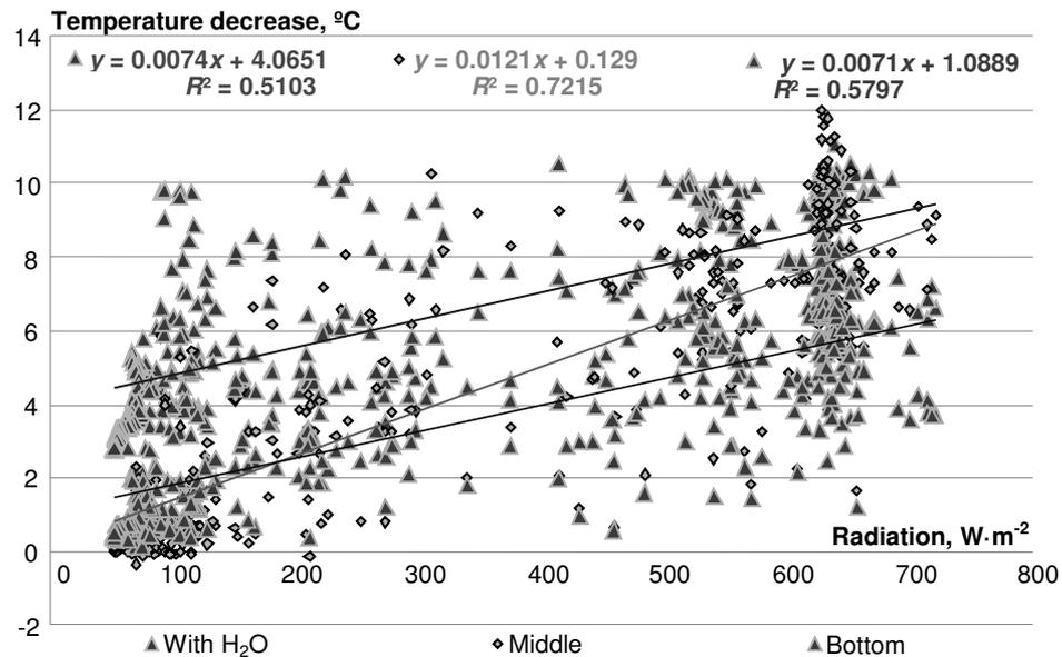
Fig. 6. Outlet atmospheric air temperatures decreases (with collector with water radiator, without radiator and absorber steel tin-plate in middle) comparing with solar radiation and temperature decrease (11:00-17:10 11.09.2012)
