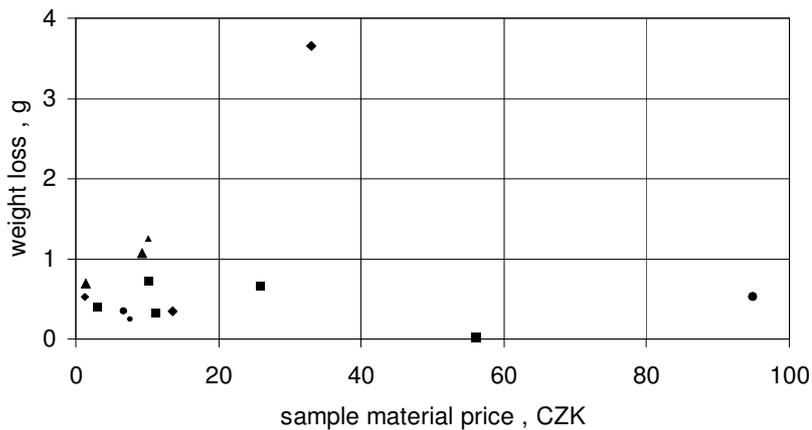
Fig. 5. Relationship between weight loss and sample price (abrasive grain size 115.5 μm)
