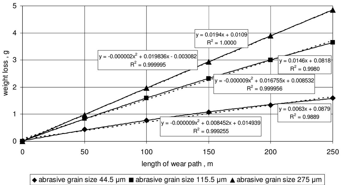
Fig. 4. Abrasive cloth abrasiveness decrease during the test (PTFE)
