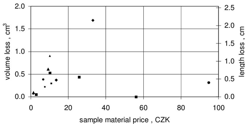
Fig. 6. Relationship between volume/length loss and sample price (abrasive grain size 115.5 μm)
