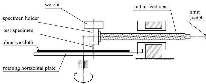
Fig. 1. Scheme of the abrasion testing machine (pin-on-disk)
