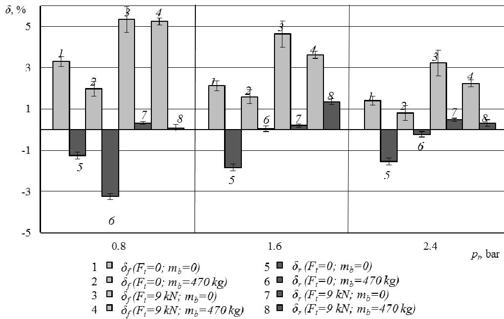
**Fig. 2. Dependence of slippage of the front  $\delta_f$  and rear  $\delta_r$  wheels of the tractor on different inflation pressure in the rear tires  $p_r$ , driving without ballast ( $m_b = 0$ ), with ballast ( $m_b = 470 \text{ kg}$ ), without tractive force ( $F_t = 0$ ), loaded with tractive force ( $F_t = 9 \text{ kN}$ ); inflation pressure in the rear tires  $p_r$ : 0.8; 1.6; 2.4 bar**
