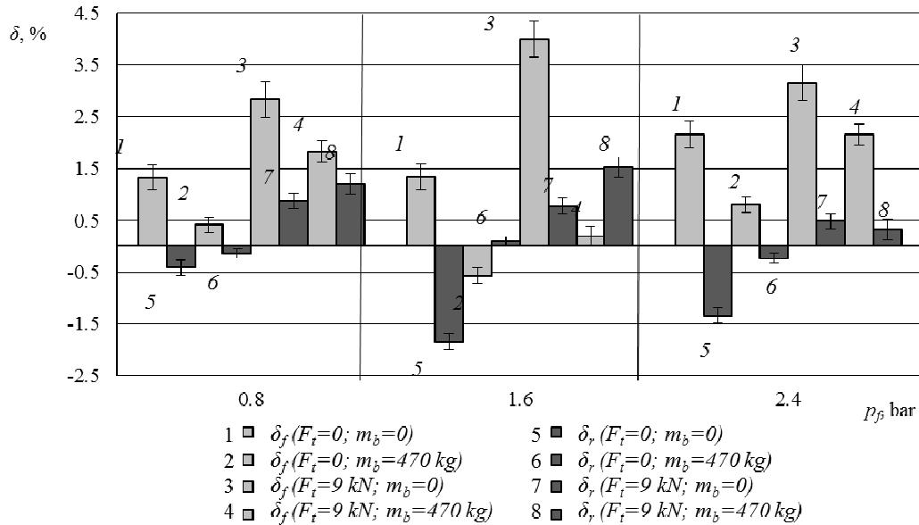
Fig. 1. Dependence of slippage of the front  $\delta_f$  and rear  $\delta_r$  wheels of the tractor on different air pressure in the front tires  $p_f$  driving without ballast ( $m_b = 0$ ), with ballast ( $m_b = 470 \text{ kg}$ ), without tractive force ( $F_t = 0$ ), loaded with tractive force ( $F_t = 9 \text{ kN}$ ); Inflation pressure in the front tires  $p_f$ : 0.8; 1.6; 2.4 bar
