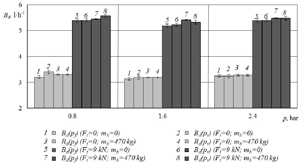
Fig. 4. Dependence on fuel consumption on different inflation pressure in the front ( $p_f$ ) and rear ( $p_r$ ) tires driving without ballast ( $m_b = 0$ ), with ballast ( $m_b = 470 \text{ kg}$ ), without tractive force ( $F_t = 0$ ), loaded with tractive force ( $F_t = 9 \text{ kN}$ ); the inflation pressure in the tires  $p$ : 0.8; 1.6; 2.4 bar
