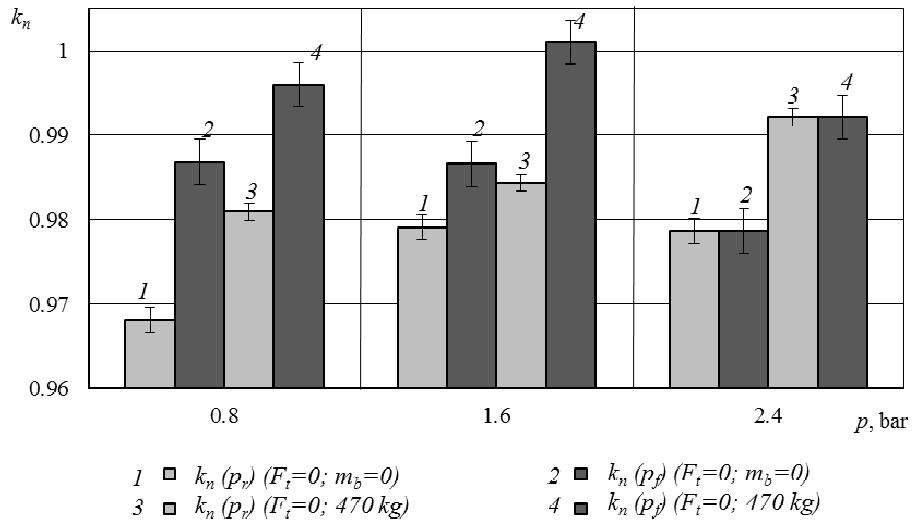
Fig. 3. Kinematic discrepancy  $k_n$  of the driving wheels of the tractor driving without ballast ( $m_b = 0$ ), with ballast ( $m_b = 470 \text{ kg}$ ) on different inflation pressure on the front ( $p_f$ ) and rear ( $p_r$ ) driving wheels: 0.8; 1.6; 2.4 bar
