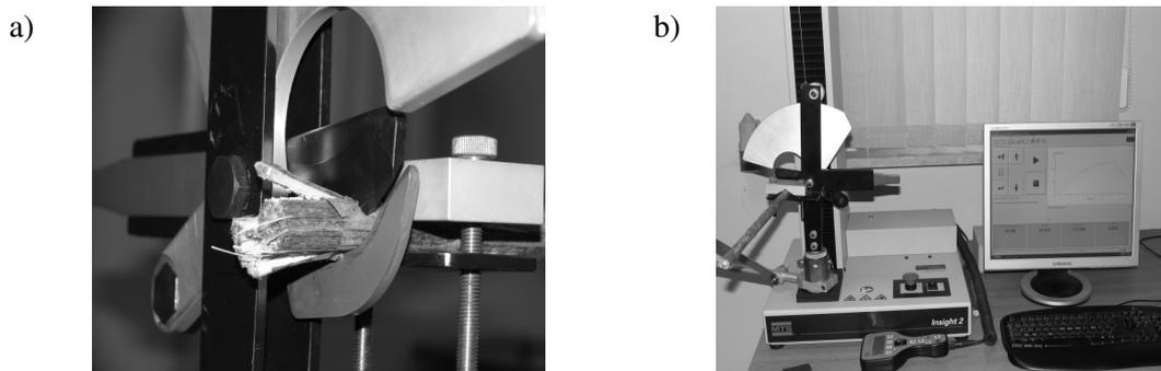
Fig. 2. Stand for determining the static work of cut plant materials: a – cutting device, b – control unit (PC) with software TestWorks 4
