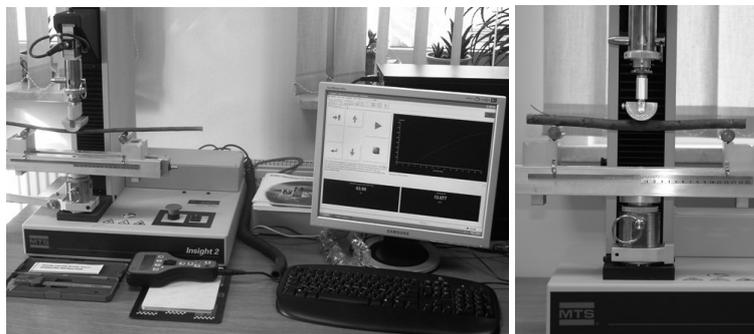
Fig. 3. Endurance machine MTS with adapter for three- point bending
