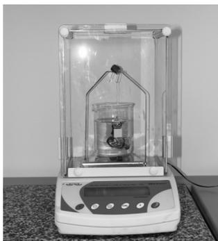
Fig. 4. Stand for determining the specific density
