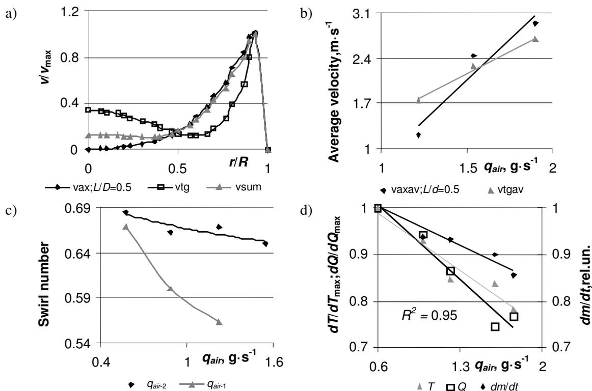
Fig. 2. Numerical estimation of the formation of the isothermal inlet flow velocity profiles (a); the effect of secondary air supply on average values of the axial and tangential velocity (b); the effect of primary and secondary air supply on the swirl number (c); the effect of secondary air supply on swirl-induced variations of the rate of thermal decomposition of wood pellets and on the main characteristics of swirling flame at thermochemical conversion of wood pellets (d)
