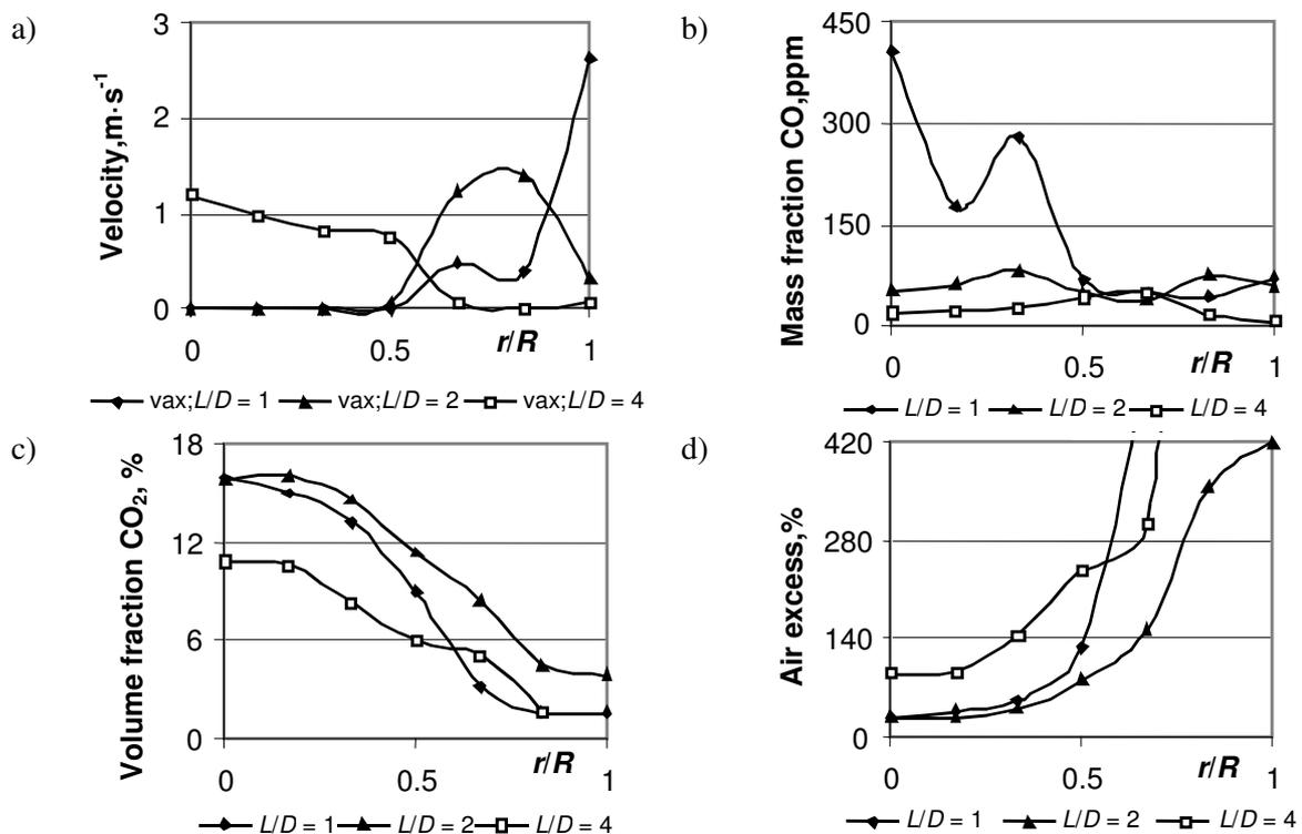
Fig. 3. Development of the flame velocity (a) and composition (b-d) profiles downstream of the swirling flame flow at swirl-induced formation of the recirculation zone at the bottom part of the combustor
