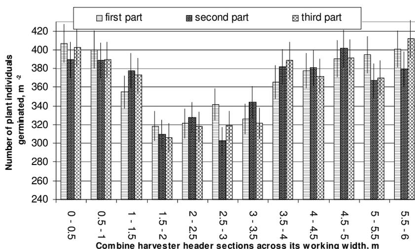
**Fig. 1. Number of plant individuals germinated at different sections across the combine harvester working width (counted 40<sup>th</sup> day after seeding, uneven placement variant, 1<sup>st</sup> trial plot divided into 3 sections)**
