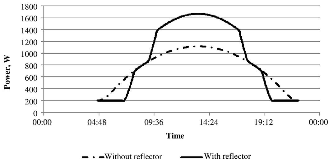
Fig. 4. Daily course of solar power received by collector with or without reflector
