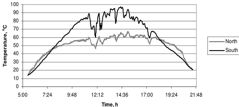
Fig. 2. Daily courses of surface temperatures at northern and southern sides of the semi-spherical solar collector, 17 June 2009 [3]
