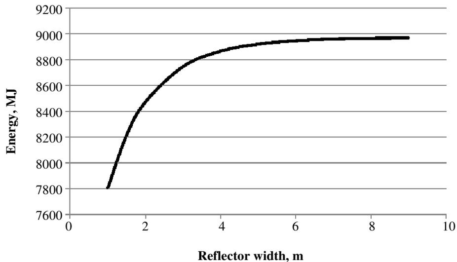
Fig. 5. Dependence of seasonal (from the 1<sup>st</sup> of March till the 31<sup>st</sup> of October) energy gain from solar collector on width of reflector
