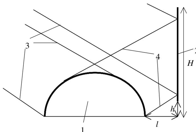
Fig. 3. Semi-spherical solar collector with reflector: 1 – collector; 2 – reflector; 3 – direct solar beams; 4 – reflected beams;  $l$  – distance between the collector and reflector;  $h$  – height of the bottom of the reflector;  $H$  – height of the top of the reflector
