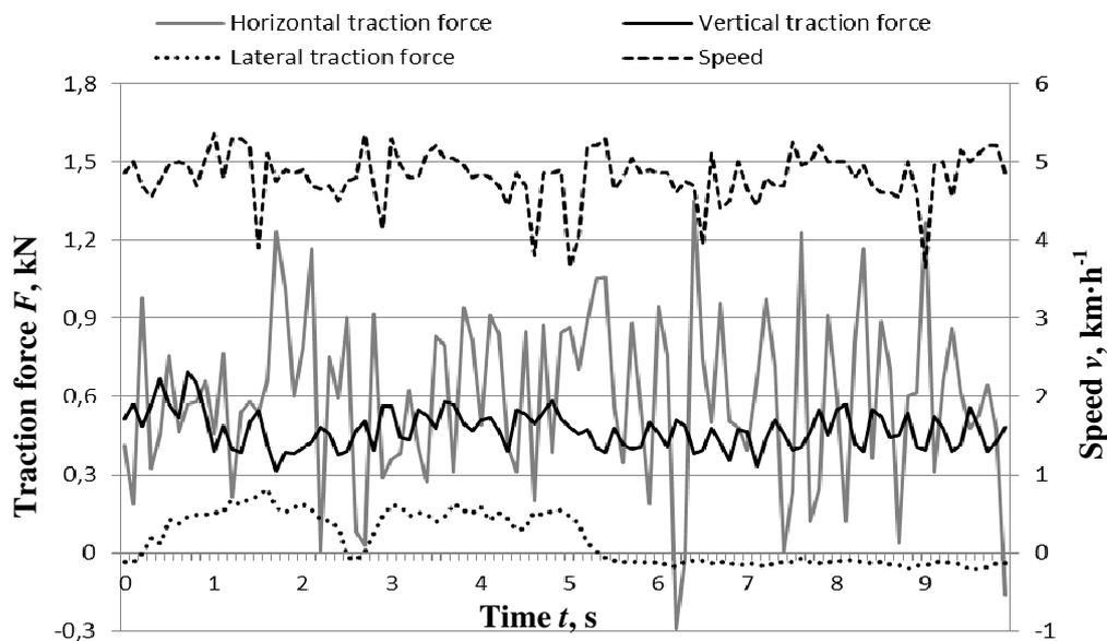
Fig. 7. Traction forces of complex coulters in the soil of 0.827 MPa hardness
