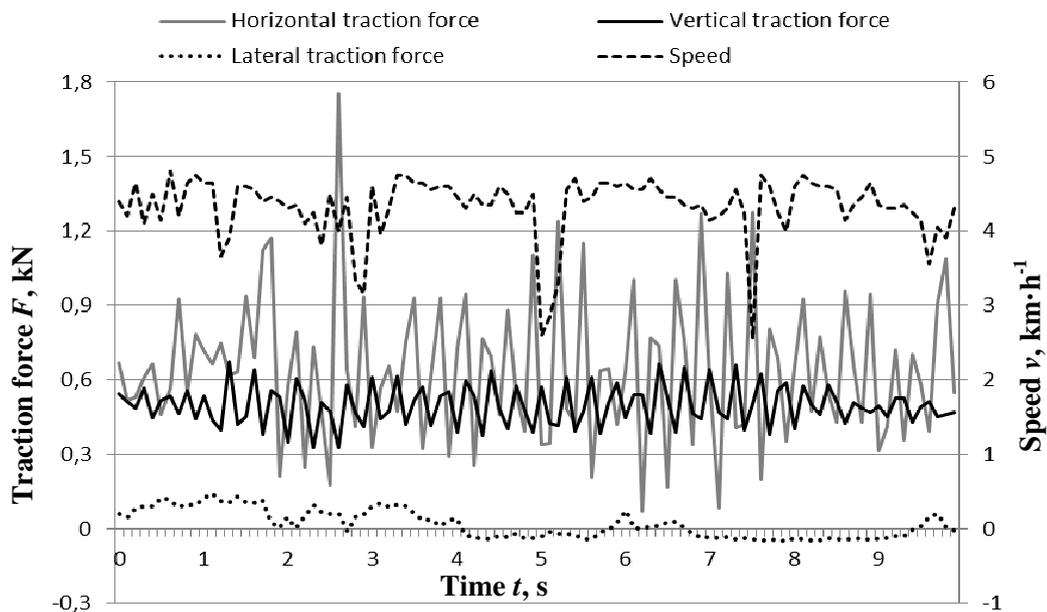
Fig. 5. Traction forces of complex coulters in the soil of 0.044 MPa hardness
