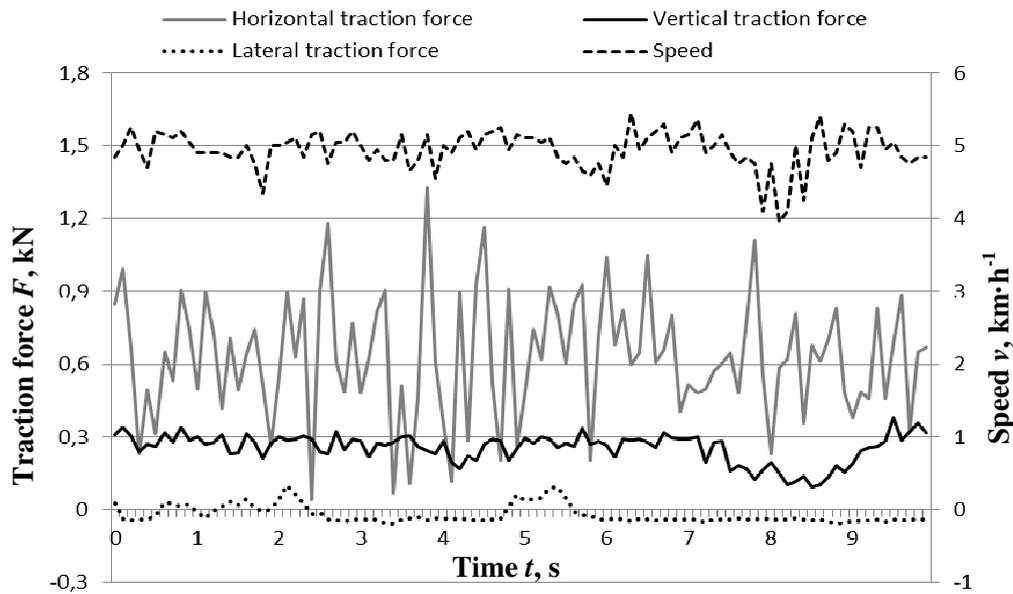
Fig. 6. Traction forces of complex coulters in the soil of 0.493 MPa hardness
