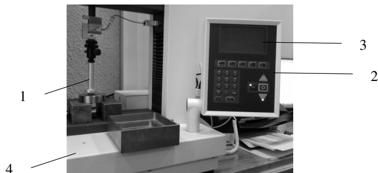
Fig. 1. Hounsfield equipment: 1 – crushing adapter; 2 – display; 3 – screen display; 4 – support of the equipment
