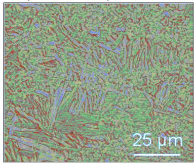
Fig.1 Initial structure of Ti-alloy, without corrosion load
