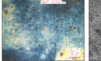
Fig. 6 Sample No. 5, 88 days of corrosion
