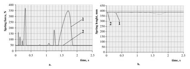
Fig. 5. Diagram of variation in time of force from spring (a) and spring length (b), for two profiles of soil surface: 1 – soil with smooth surface; 2 – soil with unevenness
