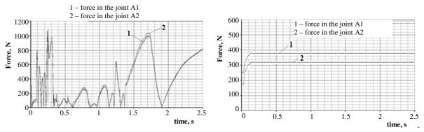
Fig. 3. Diagram of variation in time of forces from A1 and A2 joints of parallelogram mechanism (s. Fig. 2), for soil with unevenness
