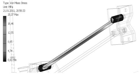
Fig. 8. Distribution of Von Mises Stress in top bar of parallelogram mechanism
