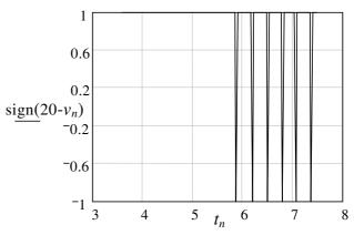
Fig. 4. " **Bang-bang**" control action in time region 3-8
