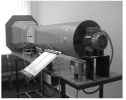
Fig. 11. Armfield wind tunnel
