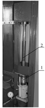
Fig. 1. Hydraulic press: 1 – press cylinder; 2 – closed die
