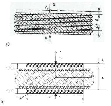
Fig. 3. Model of calculation: a - shock absorber;  $b - n^{th}$ -layer of shock absorber
