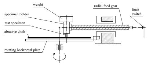
Fig. 2. Scheme of equipment for testing abrasive wear [15]
