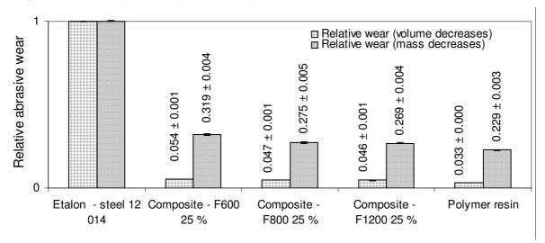
Fig. 5. Comparison of resistance against abrasive wear
