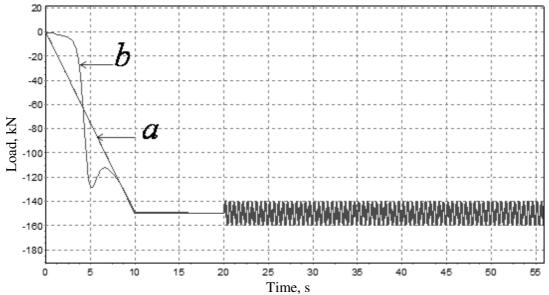
Fig. 2. Example of required (a) and implemented (b) vibropressing regimes
