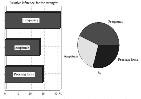
Fig. 5. Effect of vibropressing process on strength of concrete
