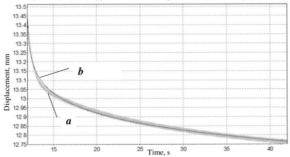
Fig. 4. Registered (a) and approximated (b) plunger displacement graph
