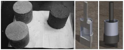
Fig. 3. Pressing plunger, mold and compacted concrete block specimens
