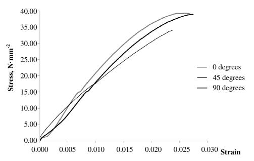
Fig. 2. The stress-strain curve of composites, reinforced by the knitted fabric
