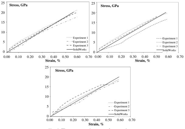
Fig. 5. The stress-strain curve of composites: (a) – direction  $0^{\circ}$ ; (b) – direction  $45^{\circ}$ ; (c) – direction  $90^{\circ}$
