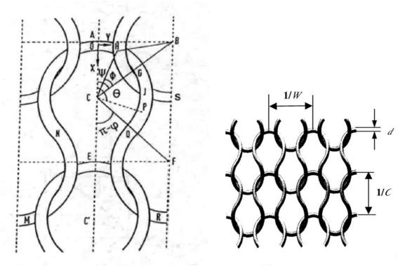
Fig. 3. Schematic presentation of the knitted fabric structure [22]
