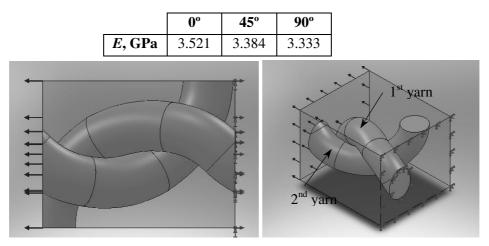
Fig. 4. SolidWorks 3D model for unit cell (knitted fabric orientation 0°)
