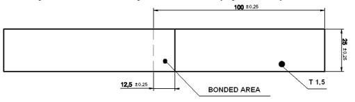
Fig. 1. Shape and dimensions of specimen - tensile shear strength
