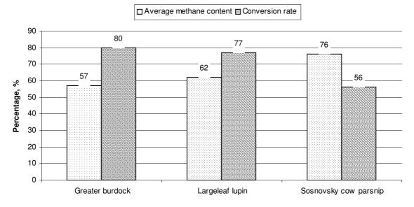
Fig. 2. Average methane content and conversion rate of organic solids
