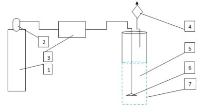
Fig. 1. Scheme of ozonation equipment: 1 – oxygen cylinder; 2 – pressure regulator; 3 – ozone generator; 4 – ozone destructor; 5 – cheese whey; 6 – diffuser; 7 – glass cylinder
