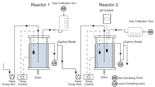
Fig. 1. Schematic diagram of two phase anaerobic bioreactor used in study
