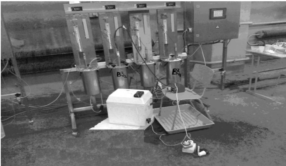
Fig. 1. Laboratory reactors, biogas yield from biomass study
