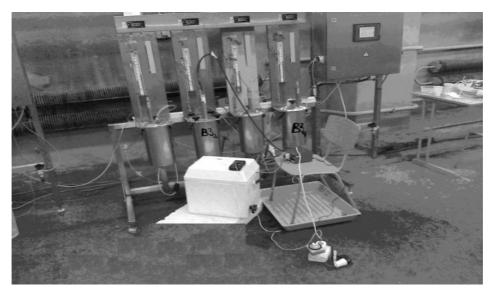
Fig. 1. Laboratory reactors, biogas yield from biomass study
