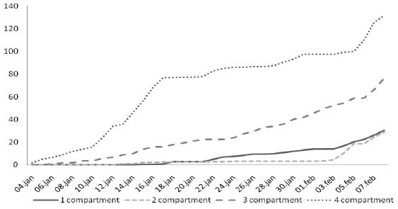
Fig. 6. Preliminary results from four stage digester for anaerobic treatment of biomass: cumulative gas evolution
