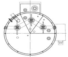
Fig. 4. Four stage digester for anaerobic treatment of biomass
