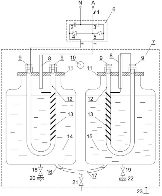
Fig 1. Water curative treatment device: 1 – auto – switch; 2,3 – condensers; 4,5 – diodes; 6 – voltage duplicator; 7 – device; 8 – isolating material pipes; 9 – metallic plates; 10 – miliampermeter; 11 – locking lids; 12 – UV bulbs; 13 – electrode; 14 – cation; 15 – anion; 16 – connecting glass pipes; 17 – hidro – seal; 18, 19, 21 – taps; 20, 22 – coal filter; 23 – metallic parts
