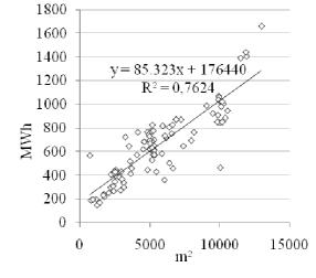
Fig. 5. Not renovated school buildings: total heat energy consumption (MWh) per annum correlation with buildings floor area  $(m^2)$
