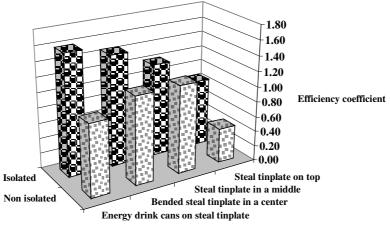
Fig. 2. Efficiency diagram of isolated and non isolated collectors
