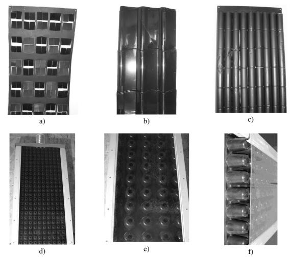
Fig. 1. Absorbers visual view: a – bended steal tinplate; b – roof material; c – energy drink cans on steal tinplate; d – 12 seed boxes in line; e – 5 seed boxes in line; f – 7 seed boxes in line
