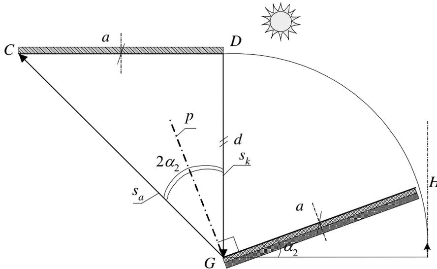
Fig. 3. Detection scheme for right mirror rotation angle  $\alpha_2$
