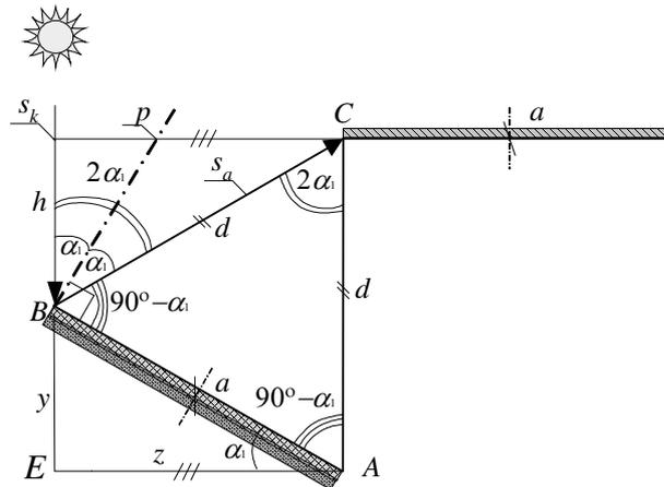
Fig. 2. Detection scheme for left mirror rotation angle  $\alpha_1$
