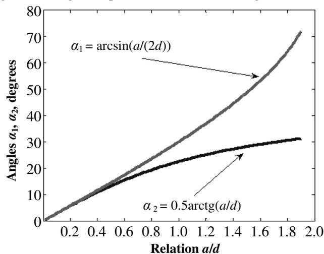
Fig. 4. Dependence of right side and left side mirror angles
