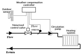
Fig. 1. Principal scheme of heating substation
