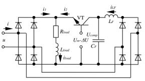
Fig. 4. Possible scheme of realization of compensation source
