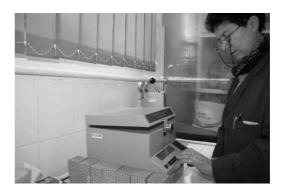
Fig. 4. Determination of calorific power
