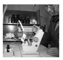
Fig. 3. Determination of refractive index
