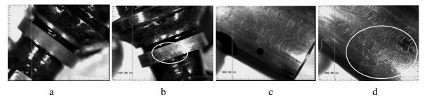
Fig. 5. Work surface of subsystem: a – unloading collar before testing; b – unloading collar after testing; c – pump plunger before testing; d – pump plunger after testing.
