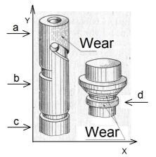
Fig. 1. Measurement methods for fuel injection pump parts [5]
