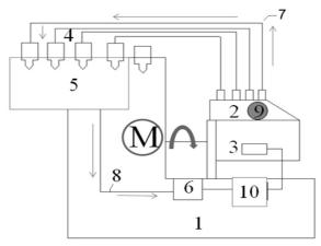
Fig. 2. Scheme of test principle: 1– stand; 2 – fuel injection pump; 3 – fuel pre-supply pump; 4 – injector; 5 – fuel container; 6 – cooling system; 7 – fuel injection pipes; 8 – fuel pre-supply pipes; 9 – thermometer; 10 – fine filter
