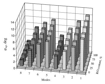
Fig. 3. Fuel injection duration in degrees of crankshaft angle as a function of performance mode and rapeseed oil content in fuel
