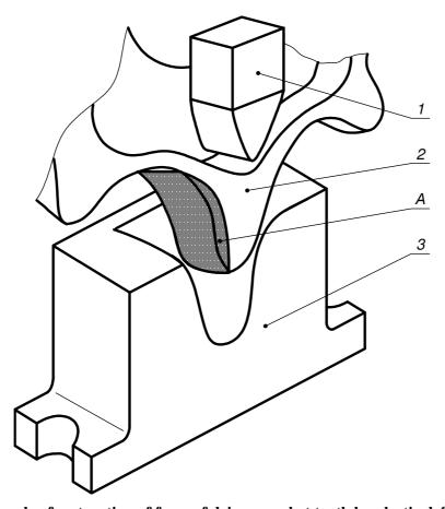
Fig. 1. Example of restoration of form of drive sprocket tooth by plastic deformation: 1 – puncheon; 2 – fragment of gear; 3 – matrix; A – demanded redistribution of volume of material
