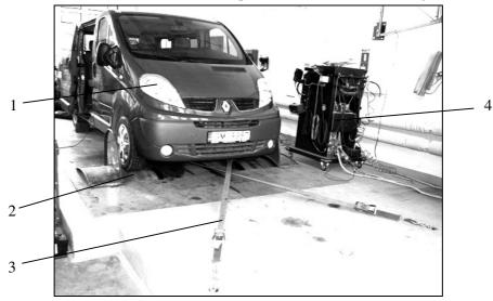
Fig. 3. **Renault Trafic on chassis dynamometer:** 1 – automobile; 2 – roll; 3 – straps; 4 – control platform
