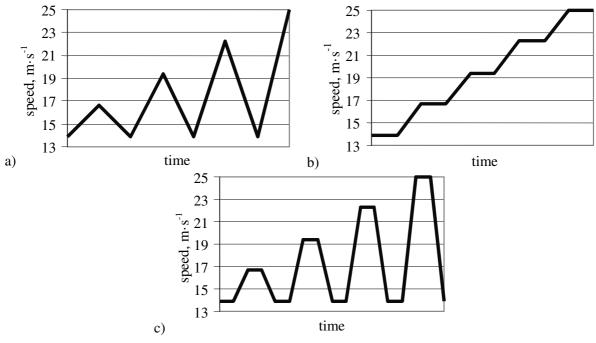
Fig. 4. Driving cycles: a – pulsing; b – gradual; c – impulse
