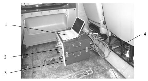
Fig. 1. AVL KMA Mobile fitted to automobile: 1 – computer for data collecting; 2 – measuring module; 3 – conditioning module; 4 – fuel supply hoses
