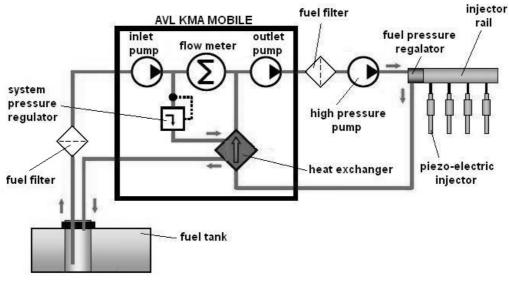
Fig. 2. AVL KMA Mobile fitting scheme [1]
